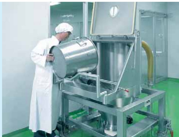
Feeding hopper with special equipment for feeding drums
