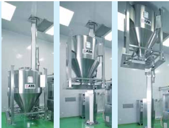
Lifting column for feeding the tablet press from BATCHTAINERS®
