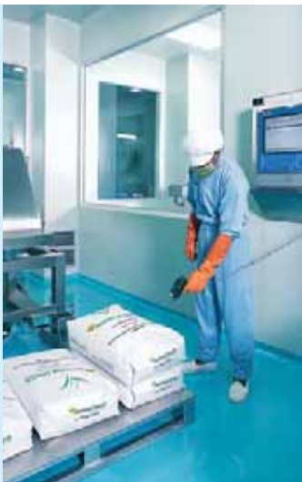
Feeding of sacks with barcode logging
