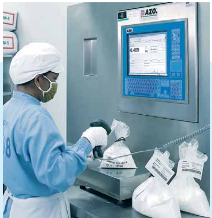
Barcode logging of the precisely weighed active ingredients
