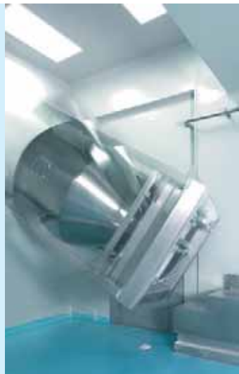
Production of a homogeneous mixture with the help of a container mixer
