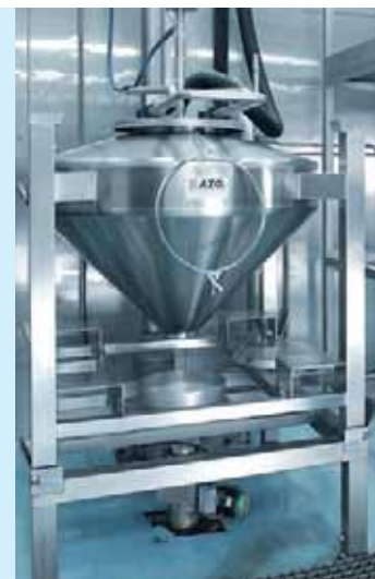
Automated container washing unit
