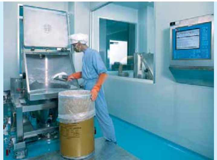
Feeding products out of drums into the closed system
