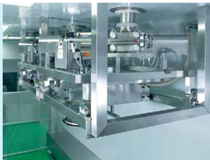
Screener with docking for metering into BATCHTAINERS®
