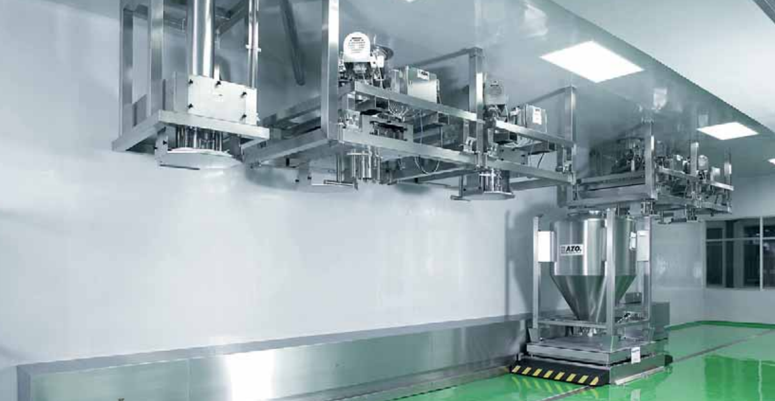
AZO COMPONENTER® for automated collection and weighing of the components
