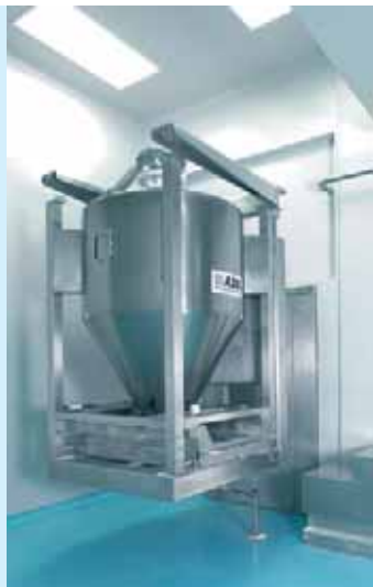
Production of a homogeneous mixture with the help of a container mixer
