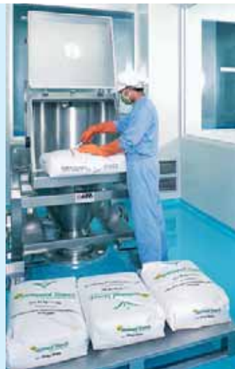
Filling sacks into the closed system
