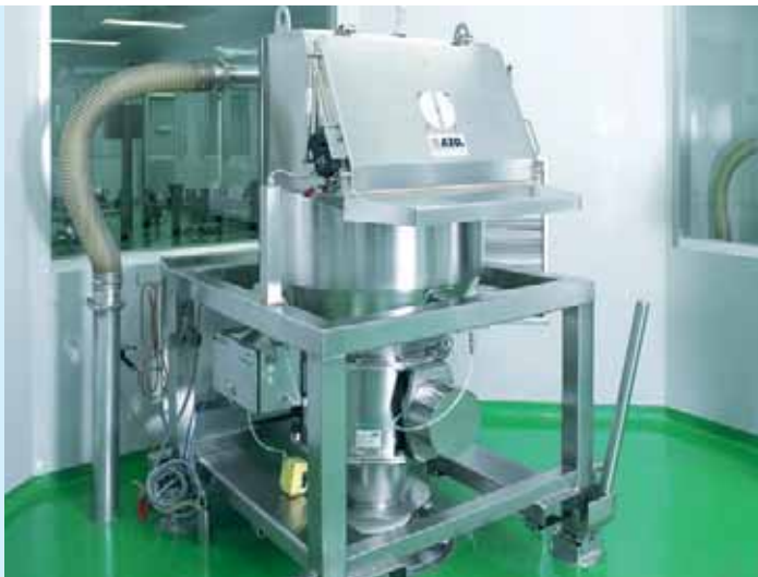
Pre-dispensing feeding hopper with lump breaker
