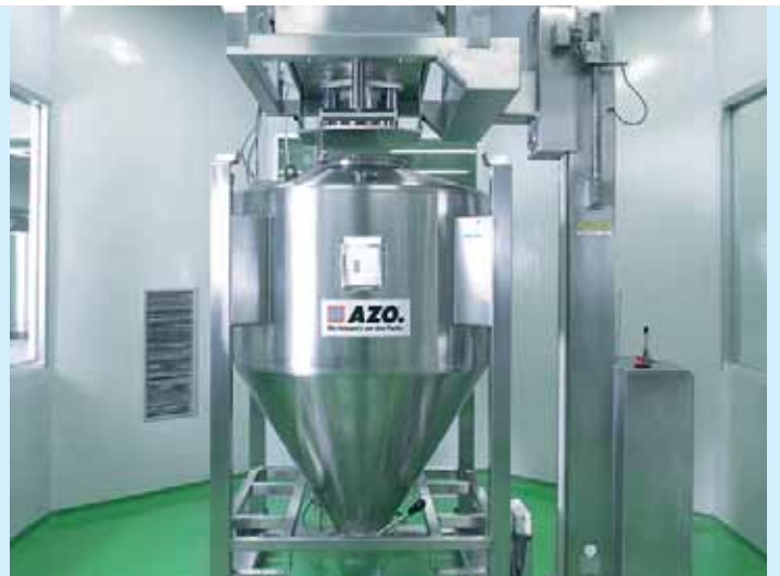
Filling the BATCHAINER® after the granulating process
