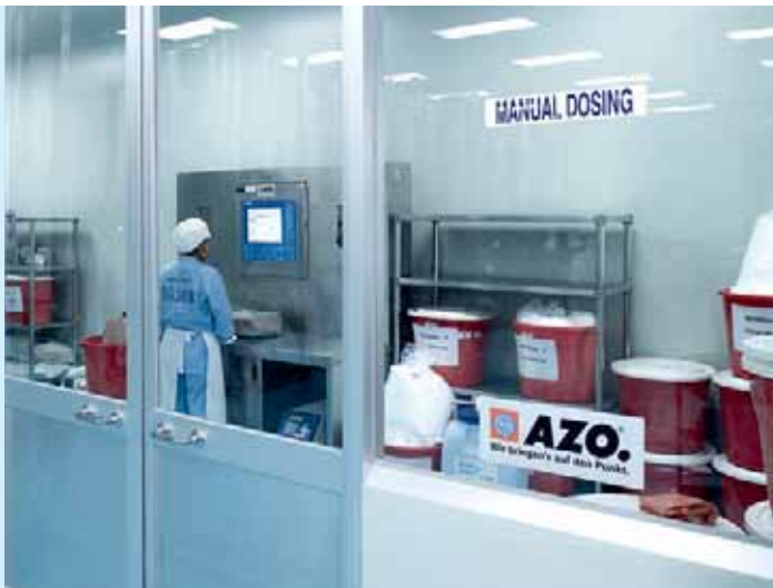
ManDos weighing system for weighing active ingredients
