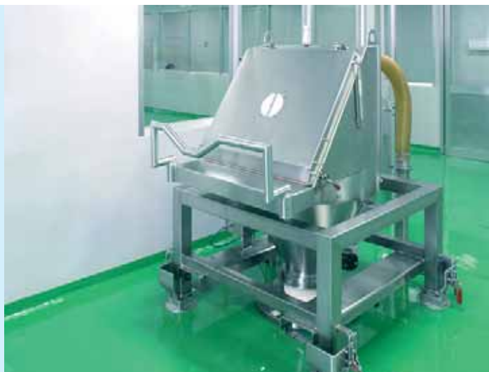
Feeding hopper for feeding sacks and drums into the closed system
