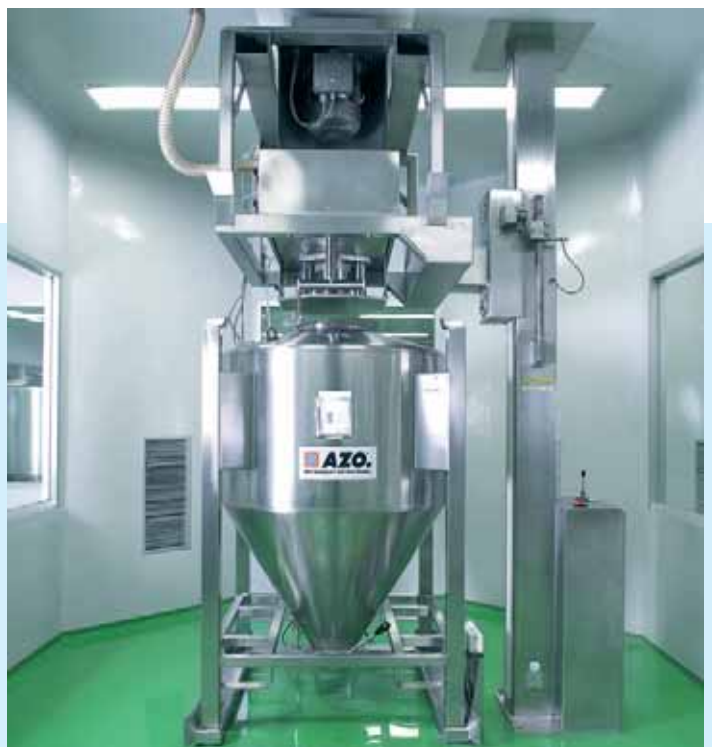
Lifting column with conical mill for feeding a BATCHTAINER®
